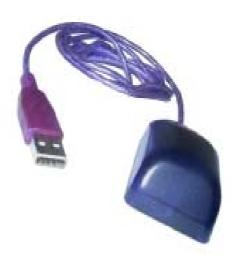
The Greenwich Instruments **USB GIrBIL** is a true IrDA USB adaptor which provides the user with a bridge to the USB port of a desktop or laptop PC, allowing transfer speeds of up to 4M bps for record synchronization, backing up and network access. As with all GIrBIL devices, no external power is required.
