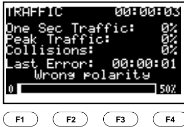
Figure 11-1. Traffic Test Results Screen (Wrong Polarity).
