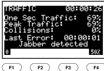
Figure 11-3. Traffic Test Results Screen (Jabber Detected).
