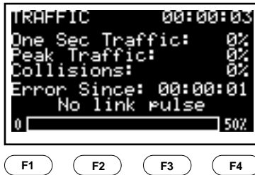
Figure 11-2. Traffic Test Results Screen (No Link Pulse).
