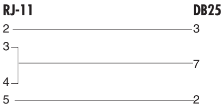
Figure A-1. Connecting a terminal, serial printer, or CPU communications port to a slave channel.
