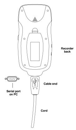
Figure 4-1. Connecting the Recorder to your PC.
