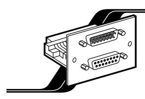
Install an Expansion Module for Matrix ServSwitch<sup>TM</sup> (our product code SW740C-R3-B) in your Switch unit to prepare that Switch to be interconnected (daisychained) with other Matrix ServSwitches in your system. Each Module has two DB15 connectors, as shown in the illustration above: The top one, IN, is female and receives video signals from other Switches; the bottom one, OUT, is male and transmits video signals to other Switches.
