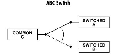
Fig. 3-1. Connections made are AC and BC — "C" is COMMON.
