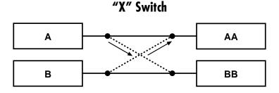
Fig. 5-1. Connections made are A-AA & B-BB or A-BB & B-AA.
