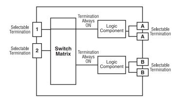
Figure 5-1. Termination configuration.
