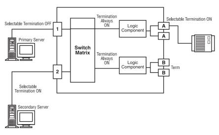
Figure 5-3. SC120A-R2 termination example 2.
