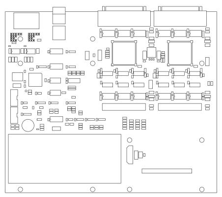
Figure 6-1. SCSI Switch component placement.
