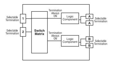
Figure 2-2. SC120A-R2 block diagram.
