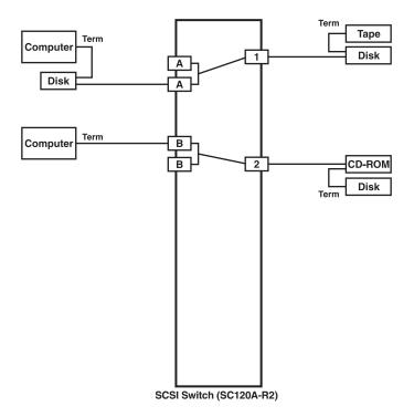
Figure 2-3. Typical switch installation.
