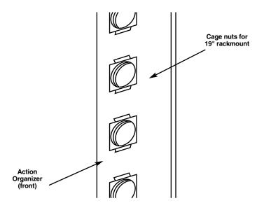
Figure 3-1. Rackmounting 19" EIA components.
