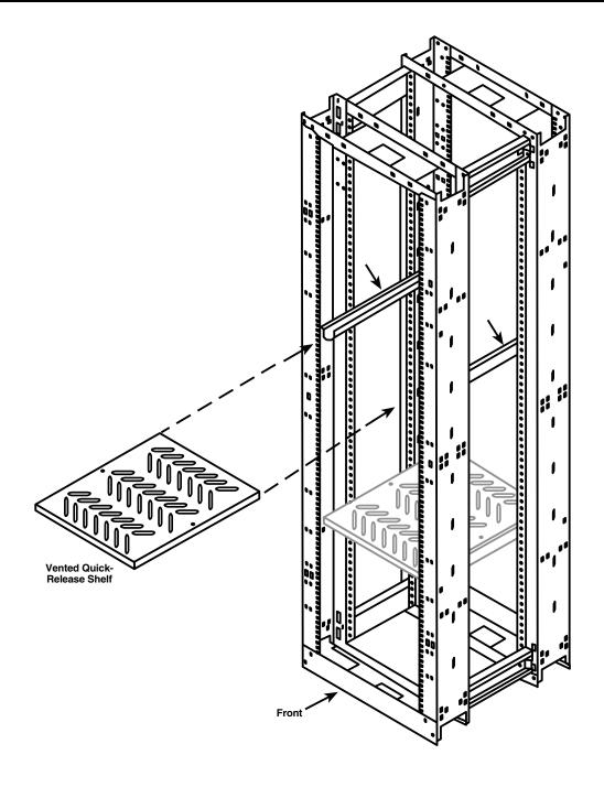
Figure 3-2. Installing the Vented Quick-Release Shelf.
