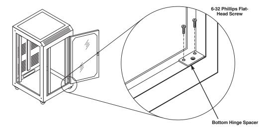
Figure 9. The bottom hinge spacer.
