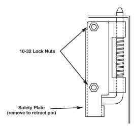
Figure 7. Remove the lock nuts.
