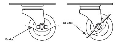
Figure 3. The brake in the off (left) and on (right) positions.
