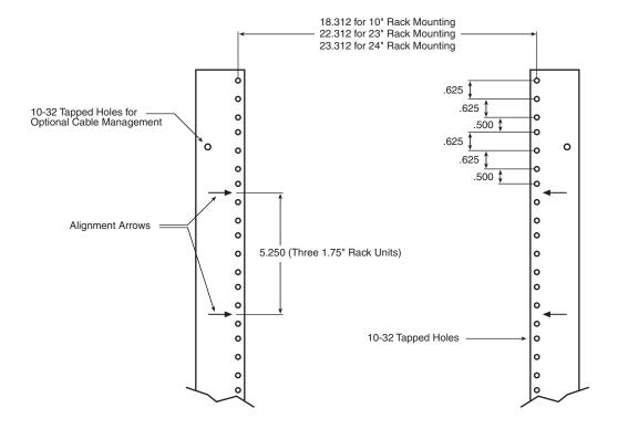
Figure 11. The mounting rails.
