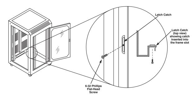
Figure 10. Relocating the latch catch.
