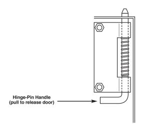
Figure 8. The hinge-pin handle.
