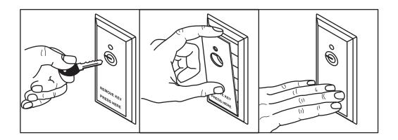
Figure 5. Opening the latch.
