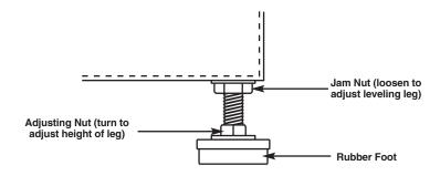
Figure 4. The Jam Nut and Adjusting Nut.
