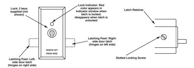
Figure 6. Front (left) and rear (right) views of the latch.
