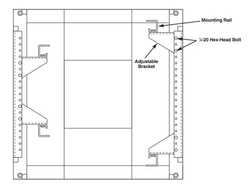
Figure 12. Adjusting the rails.
