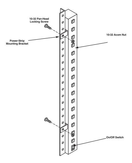
Figure 13. Installing a 16-outlet power strip.
