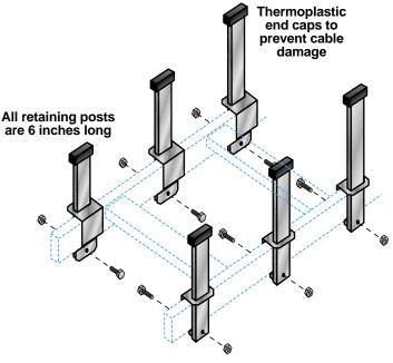
Quick assembly with a single bolt
