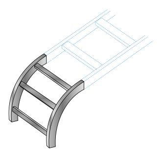
The Radius is constructed of %" x 1%" tubular steel. It has an outside corner bend width of 12" and a 33° angle between stringers.
