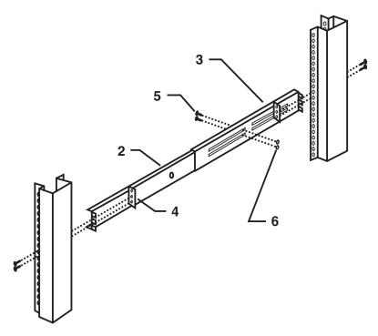
Figure 3-14. Installing the Rear Brackets on the Slides and Attaching the Slides to the Corner Posts.
