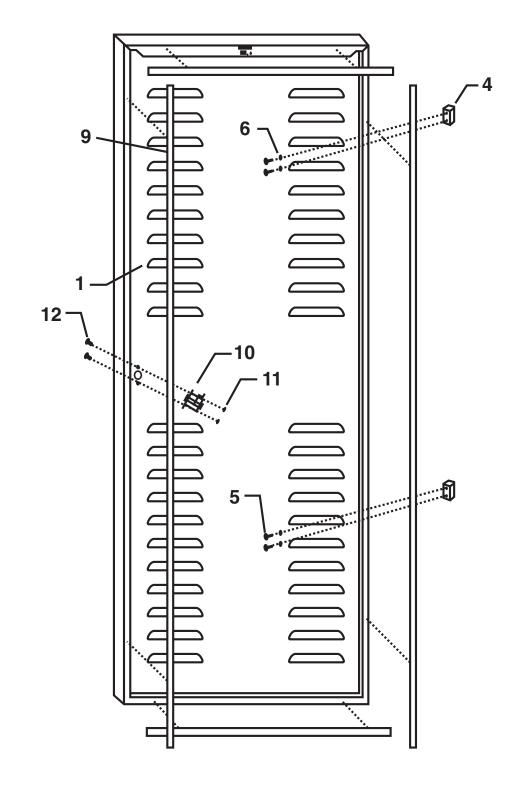
Figure 3-5. Installing the Short Steel Door.
