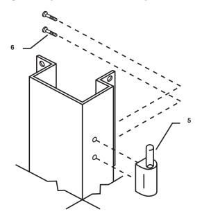
Figure 3-4. Installing Hinges on the Corner Post.
