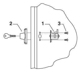
Figure 3-7. Installing the Lock—Steel Door Only.
