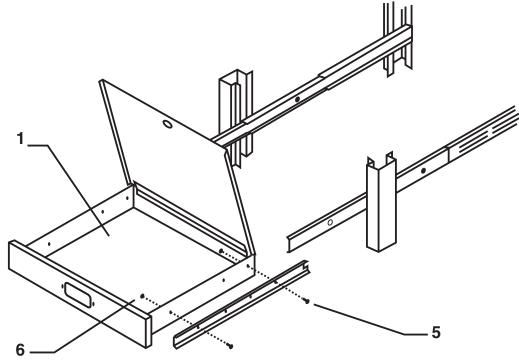
Figure 3-15. Assembling the Drawer.
