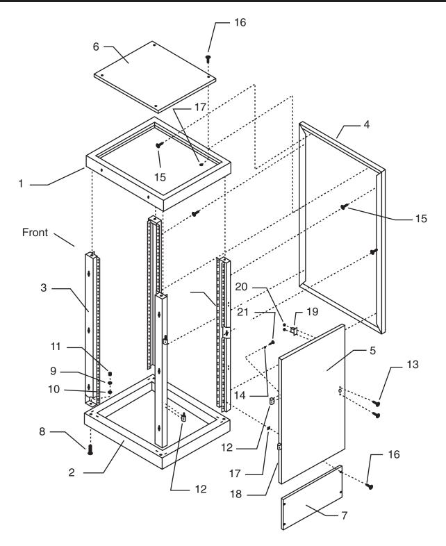
Figure 3-3. Assembling the Comm Cabinet.
