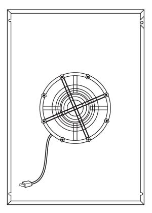
Figure 3-11. Fan Assembly.
