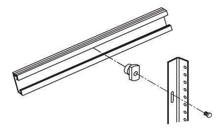
Figure 3-2. Assembling the Vertical Tapped Mounting Rails.
