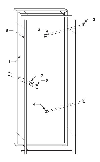
Figure 3-6. Installing the Standard Steel Door.
