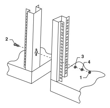
Figure 3-18. Assembling the Joining Kit.
