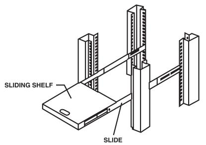
Figure 3-17. Attaching the Sliding Shelf.
