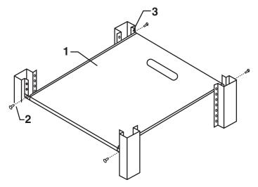
Figure 3-8. Installing the Solid or Vented Shelf.
