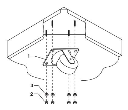
Figure 3-13. Installing the Casters.
