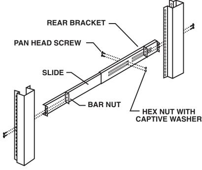
Figure 3-16. Attaching the Slide to the Rear Bracket.
