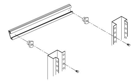
Figure 3-1. Assembling the Horizontal Mounting Rails.
