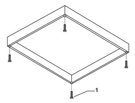
Figure 3-12. Installing the Leg Levelers.
