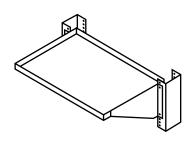
Figure 6. Shelf can be inverted to make a ¾" deep tray.
