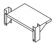
Figure 2. Shelf front flush to rack front.
