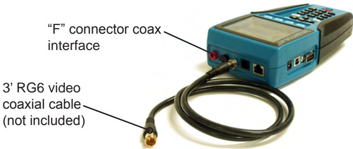
Figure 4. Video Coaxial Cable Connected to Validator-NT
