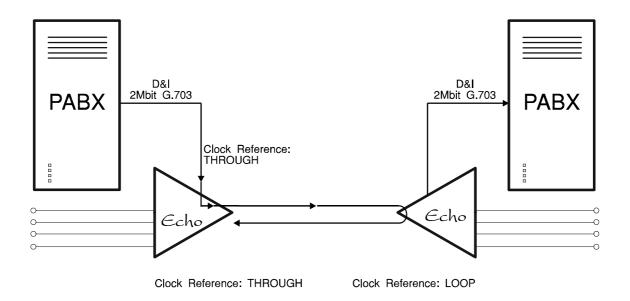
In this example, the master clock is derived from the PABX which is connected to the D&I channel.
