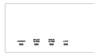
When the multiplexer is un-connected or has lost carrier, the CARRIER LED will flash slowly. A faster flash shows that CRC4 sync hunt mode has been entered.
