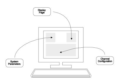
Upper left -**System parameters** (Mode, Clock Ref, Carrier, Idle Bandwidth, and Configure etc.).
