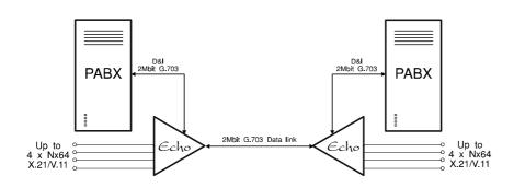
The Echo is set so that the slots used by the PABX are passed through to the main G.703 link transparently. This is described on page 15. The remaining unused timeslots can now be assigned as required to the channel ports.
