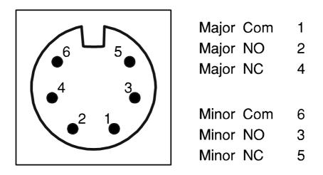
Note that the contacts are **not** mechanical, and have an internal resistance of around 100 Ohms. This should be considered when making a connection to external equipment.
