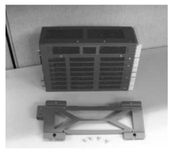
5. Slide the Unit into rack mounting bracket.
