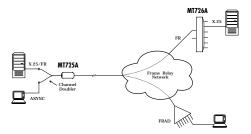
Figure 2-2. Fradswitch-2 A/S using channel doubler cable for local configuration or additional async access channel. (FR=Frame Relay.)
