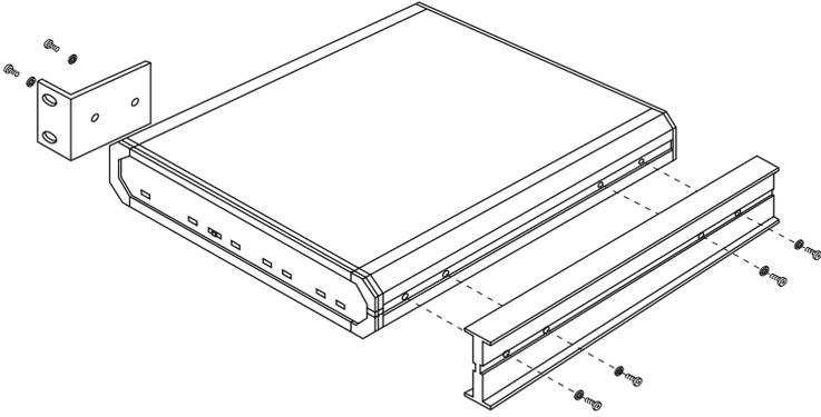
**Figure 3-3. Attaching the rail and bracket to one of the two FOLDS.**
