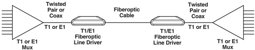
Figure 2-1. FOLD-and-mux application.
