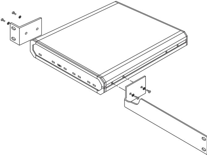
**Figure 3-2. Putting together the rackmount assembly for a single FOLD.**
