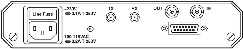
Figure 3-5. Rear panel of the AC-powered FOLD models.
