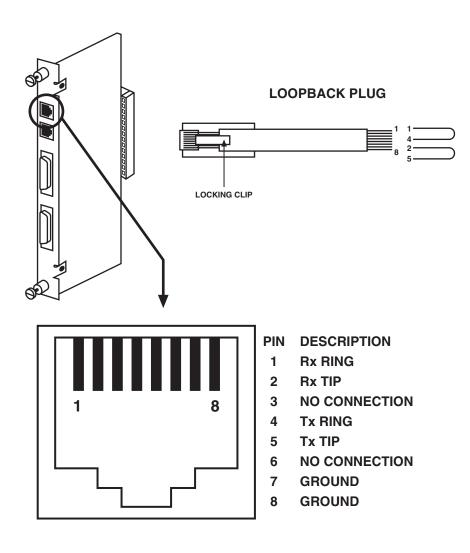
Figure 2-4. NET Interface Pinout.
