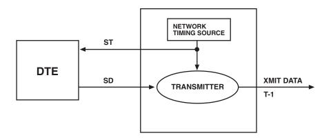
Figure 4-6. Loop 2 Timing Diagram.
