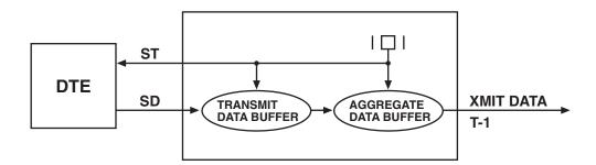
Figure 4-2. Internal (Master) Crystal Timing Diagram.
