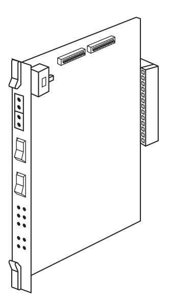
Figure 2-1. T1 CSU/DSU Card.
