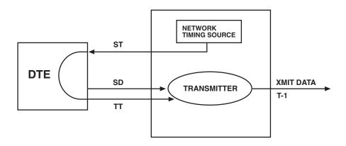
Figure 4-5. Loop 1 Timing Diagram.
