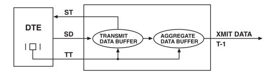
Figure 4-4. External Channel Timing Diagram.
