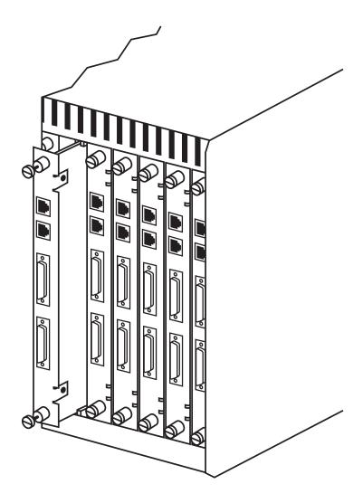
Figure 3-2. Installing the I/O Interface Module.
