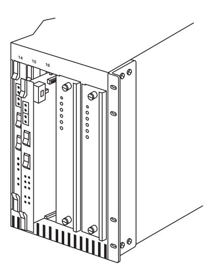
Figure 3-1. Installing the T1 CSU/DSU Card Module.
