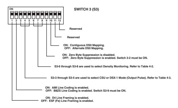
Figure 4-1. Configuration DIP Switches.
