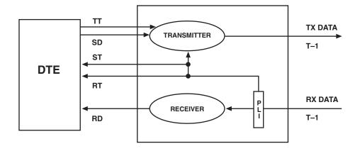
Figure 4-3. Loop (Slave) Timing Diagram.
