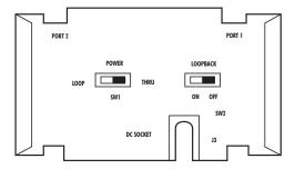
Figure 3-1. Strapping Diagram.
