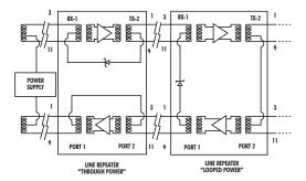
Figure 3-2. Telco Simplex Power Arrangement.
