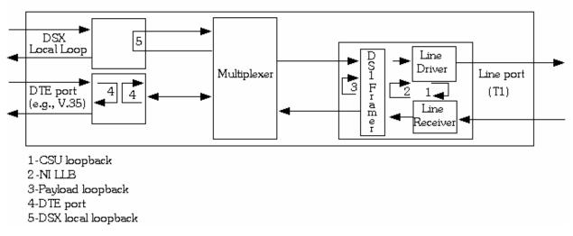
Figure 4-1 Loopback Block Diagram
