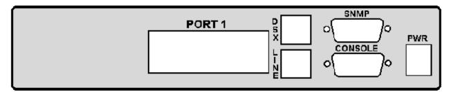
Figure 3-1 SNMP Connection
