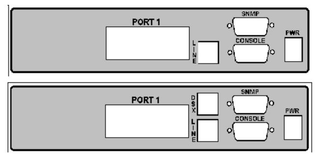
Figure 2-2 1510 CSU/DSU Rear Panel - Two Versions Shown
