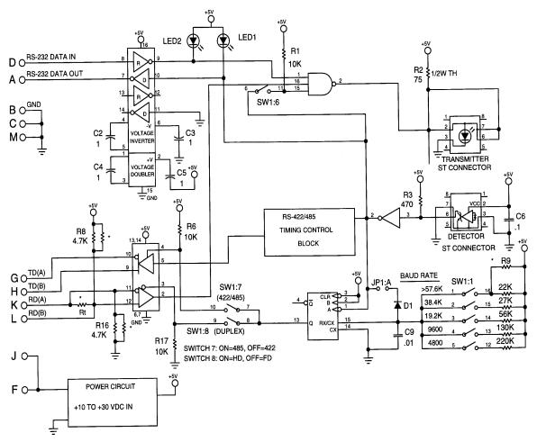
Figure 4: MED100A Circuit Diagram
