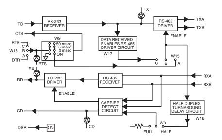
Figure 3-2. Simplified Functional Block Diagram (DCE Operation).
