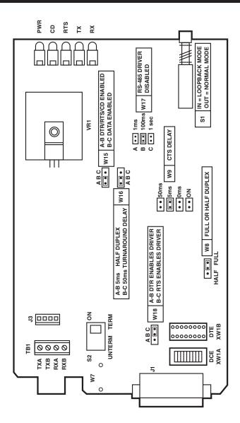
Figure 3-1. PCB Layout.
