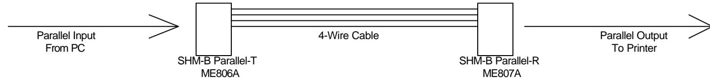
The SHM-B Parallel-T accepts parallel data from the PC, converts it to serial data, and sends the serial data over twisted-pair cable to the SHM-B (serial). The Serial SHM-B receives the serial data, converts it to RS-232 specifications, and sends the data to the RS-232 serial printer.
