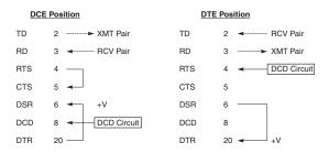
Figure 3-3. DCE/DTE Switch Configuration.
