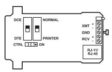
Figure 3-4. Strapping Diagram.
