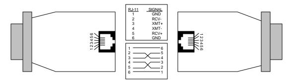
If there is a shield around the telephone cable, it may be connected to "G" (GND)on the RJ-11 connector. To avoid ground loops, we recommend connecting the shield at the computer end only. A ground wire is not necessary for proper operation of the Mini Driver
