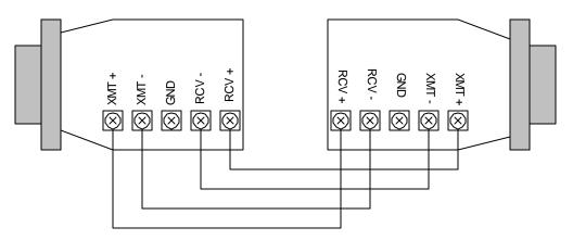
If there is a shield around the telephone cable, it may be connected to "G" on the terminal block. To avoid ground loops, we recommend connecting the shield at the computer end only. A ground wire is not necessary for proper operation of the Mini Driver MP9.
