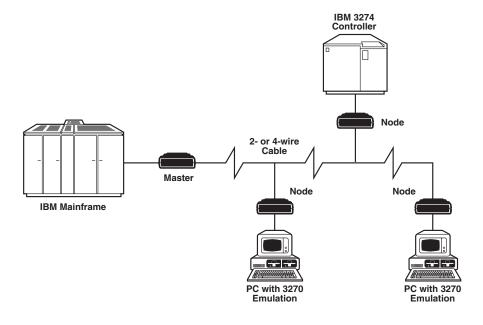
Figure 2-2. Multipoint Synchronous Application.
