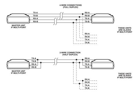
Figure 3-1. Inter-Connect Wiring Diagram.
