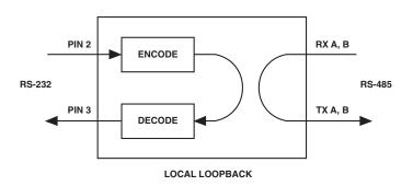
Figure 5-1. Line Loopback Test.
