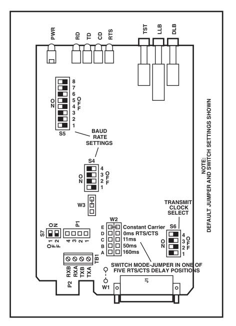
Figure 3-2. Printed Circuit Board Layout.
