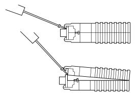
When the unit is open, you'll be able to see terminal blocks located at the rear of the PC board.
