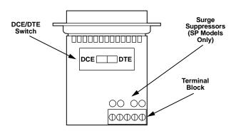
Figure 3-1. Location of the DCE/DTE switch.
