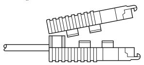
11. Insert one captive screw through a saddle washer and then insert the captive screw with the washer on it, through the hole in the DB25 end of the case. Snap that side of the case closed. Repeat the process for the other side.
