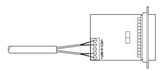
8. Place the two halves of the strain-relief assembly on either side of the telephone wire and press together lightly. Slide the assembly so that it is about two inches (5 cm) from the terminal posts and press together firmly.
