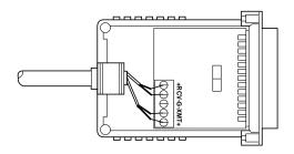
10. Bend the top half of the case as necessary to place it over the strain relief assembly. Do not snap the case together.
