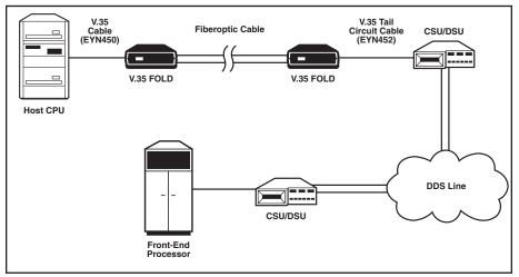
Figure 7. V.35 FOLD tail-circuit application.
