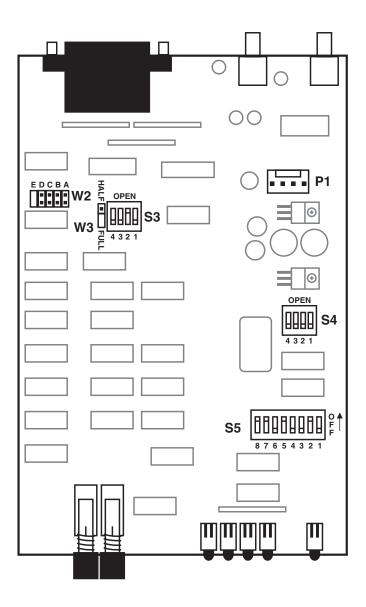
Figure 2. Circuit Board Layout for the V.35 FOLD.
