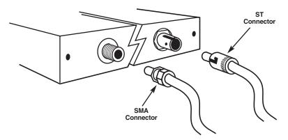
**Figure 5. Fiber Optic Connectors**
