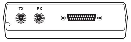
Figure 3. The rear panel of the V.35 FOLD.
