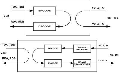
Fig. 6.1. Line and Digital Loopback Schemes
