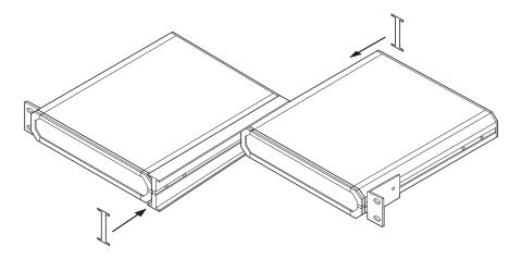
Figure 4-3. Fastening the two LHM-19.2s together.
