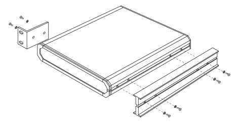
Figure 4-2. Preparing each LHM-19.2 for dual rackmounting.
