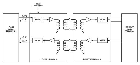
Figure 6-4. Remote digital loopback.
