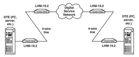
Figure 2-2. Four LHM-19.2s in a tail-circuit application.
