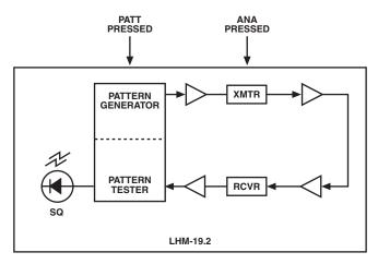
Figure 6-1. Single-modem BERT during local analog loopback.
