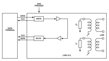
Figure 6-3. Local analog loopback.
