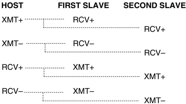
**Figure 4-2. Two-pair wiring for host and slave A/SLDs.**
