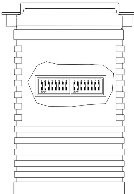
**Figure 3-1.** The A/SLD's internal configuration switches.
