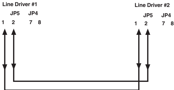
Figure A-5. Two-wire hook-up point-to-point.
