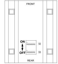
Figure 4. Underside of Compact mDSL Modem, showing location of DIP switches
