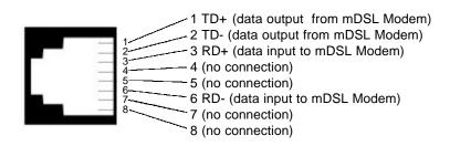
Figure 7. mDSL Modem 10BaseT Ethernet RJ-45 Connector Pinout
