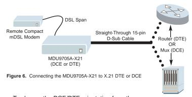
To change the DCE/DTE orientation from the default position (DCE), you must open the case Compact mDSL Modem case.
