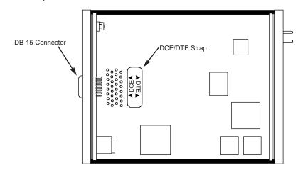
Figure 8. Setting the DCE/DTE Strap
