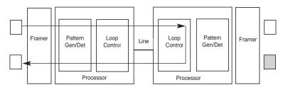
Figure 16. Block Diagram Remote Loop
