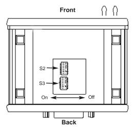
Figure 1. Underside of Compact mDSL Modem, Showing Location of DIP Switches
