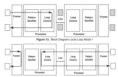
Figure 14. Block Diagram Local Loop Mode 2
