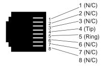
Figure 11. mDSL Access Rack Card twisted pair line interface.
