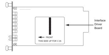
Figure 3. Close up of Top Side of mDSL Access Rack Card Interface Driver Board
