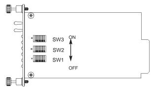
Figure 1. mDSL Access Rack Card, showing configuration switches and interface board
