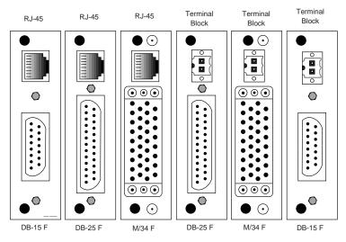
Figure 5. mDSL Access Rack Card interface card options
