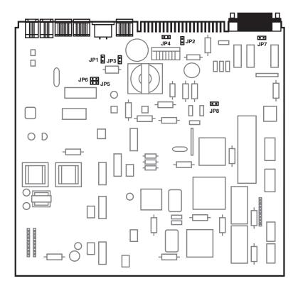
Figure D-1. Modem Circuit Board—Jumper Locations.
