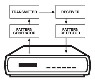
Figure 7-4. External Analog Loopback Self Test (ALBST).
