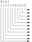
Pulse dialing rate (pulses per sec): 0=10, 1=20 Wait for carrier (sec): 0=30, 1=45, 2=60, 3=75 T1 timer (sec): 0=0, 1=0.3, 2=0.8, 3=1.6, 4=3.0 Carrier detect level, dial (dBm): 0=-26,1=-33, 2=-43 TX level, dial: 0=permissive, 1=programmable Disconnect, RTS (sec): 0=off, 1=140, 2=120...7=20 Disconnect, line current: 0=disable, 1=enable Disconnect, carrier: 0=disable, 1=enable Disconnect, TX space: 0=disable, 1=enable Disconnect, RX space: 0=disable, 1=enable Auto-answer: 0=disable, 1=enable
