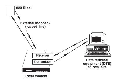
Figure 7-3. External Analog Loopback Test (ALBX).
