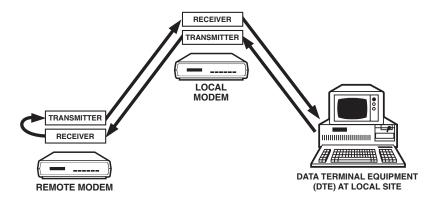
Figure 7-5. Digital Loopback Test (DLB).
