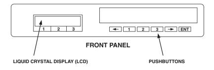
Figure 2-2. Front-Panel LCD and Controls.
