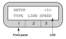
The SETUP menu has six screens. Use the arrow pushbuttons until the option you wish to configure is displayed on the bottom line of the LCD window. Select the option you wish to configure by pressing the pushbutton that corresponds to the number on the front panel.
