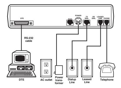
Figure 2-1. Modem 34336 Connections.
