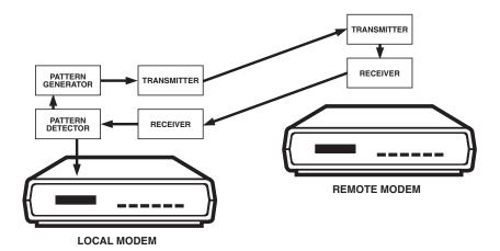
Figure 7-7. Remote Digital Loopback Self Test.
