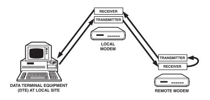
Figure 7-6. Remote Digital Loopback Test (RDL).
