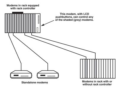
Figure 4-1. Remote control-address control mode.
