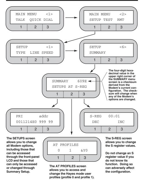
Figure C-1. How to access the Summary-Setup Screens.
