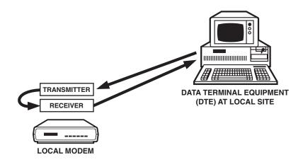
Figure 7-1. Analog Loopback Test.
