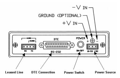
Figure 2-3. Transmission Line Interface
