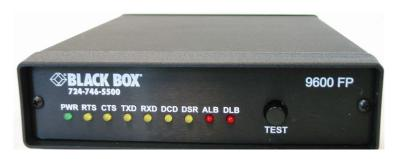
Figure 2-2. Front View of the Modems
