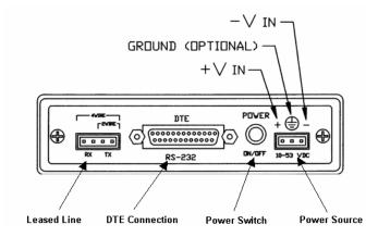
Figure 2-1. Back View of the Modems
