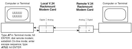
Figure 6-3. Digital Loopback Test (remote/automatic).
