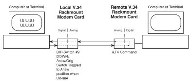
Figure 6-6. Digital Loopback Test (remote/automatic, Synchronous).
