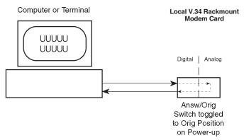
Figure 6-4. Local Analog Loopback Test (Synchronous Mode).
