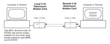
Figure 6-2. Digital Loopback Test (local/manual).
