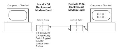
Figure 6-5. Digital Loopback Test (local/manual, Synchronous).
