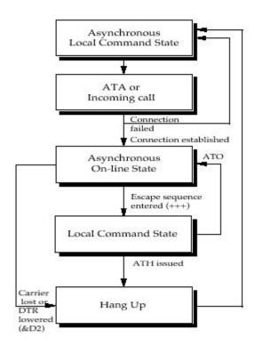
Your modem is pre-configured to automatically answer any incoming call, provided it is switched on, is in local command state, DTR is high and is not performing a test. If you receive a call on the phone line the modem is connected to, it will answer the call and attempt to connect to the calling modem.
