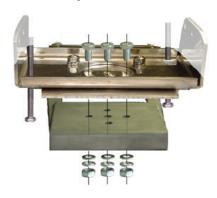
Your **Black Box LWU** head can be fixed to its stand with the three M6x25 bolts. On the figure you can see a plinth of a **Black Box LWU** unit, a head of a **Black Box LWU**mounting bracket, and the necessary fixing parts. The steps of the fixing are:
