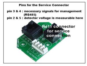
Using the RJ11 Service Connector you can connect your management indoor unit to the head.
