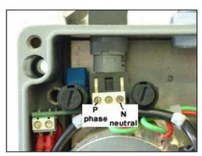
For the power connection recommended to use three-wired Ø0,75mm cables. The order of the connection can be seen on the figure.
