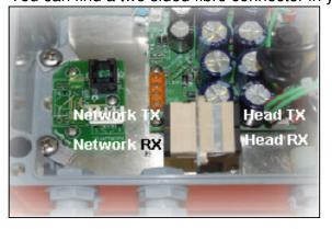
cable of your head into the one side of the connector, and into the other side you have connect the fibre cable of you network equipment (switch; router or LB combiner). The fibre plugs of the heads are always SC typed, which means that them cross-sections are cubic form. The fibre connector in the ODIU is SC-SC typed, so you have to provide an SC fibre plug for you network. The SC-SC connector is a reversible part, so you can connect in the first plug where you
