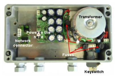
The ODIU made from poly-propylene enforced with fibre. This construction provides robust shock and waterproof environment (IP65) for the electrical devices.
