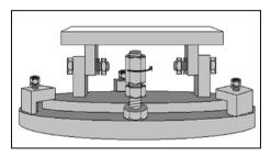
Open the spacers until it reaches the bottom of the upper plate of the ABU. Repeat this on the back side too.
