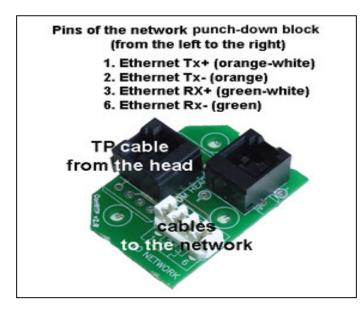
You can find a TP connector unit in your ODIU, with there connectors. You have to plug in the TP cable of your head into the RJ45 connector. network is connectable to the LB system using the white one rowed connector, where you have to connect the four cable of your network with the help of the punch down tool. The order of the cable can be seen on the figure.
