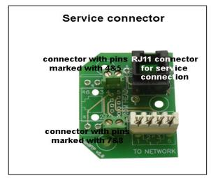
Using the RJ11 Sevice Connector and the two green connectors you can connect your management indoor unit to the head.
