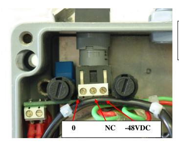
The wrong polarity of the cables can damage the power supply.
