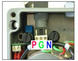
For the power connection recommended to use three-wired  $\emptyset$ 0,75mm cables. The order of the connection can be seen on the figure.
