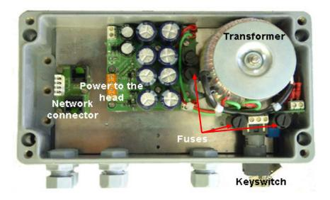
The ODIU made from poly-propylene enforced with fibre. This construction provides robust shock and waterproof environment (IP65) for the electrical devices.
