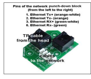
You can find a TP connector unit in your ODIU, with there connectors. You have to plug in the TP cable of your head into the RJ45 connector. Your network is connectable to the LB system using the white one rowed connector, where you have to connect the four cable of your network with the help of the punch down tool. The order of the cable can be seen on the figure.
