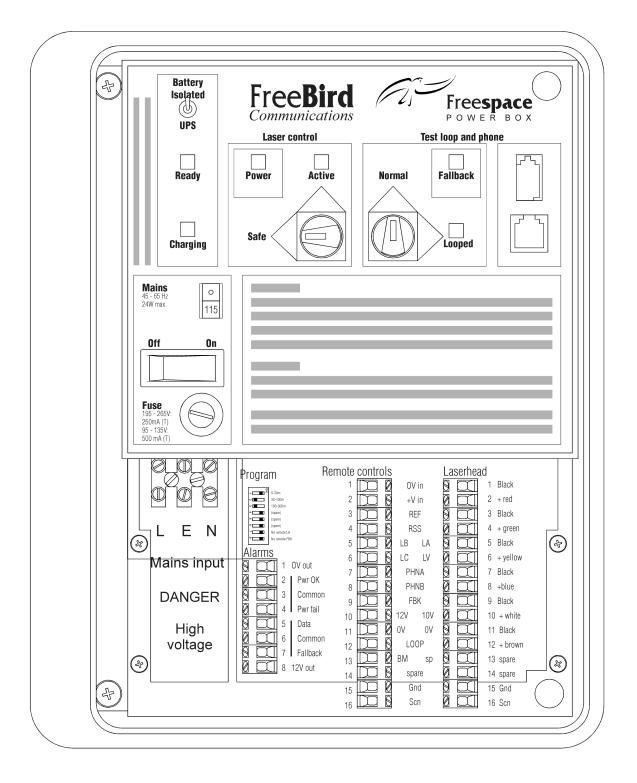
Figure 3-4. Power Box Front Panel.
