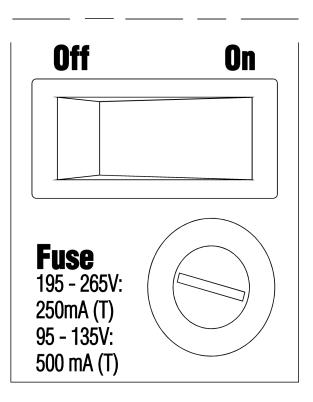
Figure 3-6. Fuse Assembly and Mains Rocker Switch.
