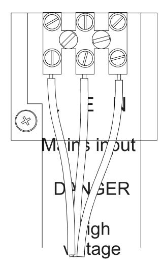
Figure 5-4. Utility Power Connection Terminations.
