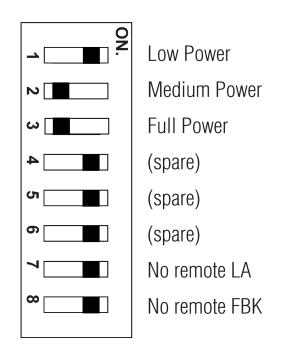
Figure 3-7. Program DIP Switches.
