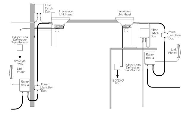
Figure 3-1. Typical Freespace Turbo Installation.
