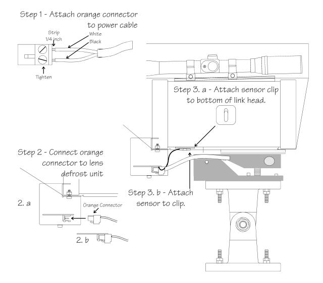
Figure 5-7. Lens Defroster Power Connection.
