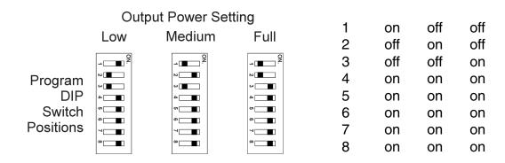
Figure 5-9. Program DIP Switch Positions.
