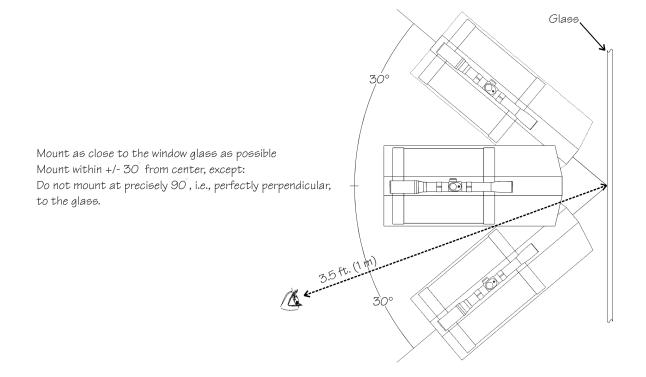
Figure 3-11. Mounting Link Heads Indoors.
