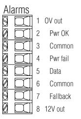
Figure 3-9. Remote Control Connection Block ("Alarms").
