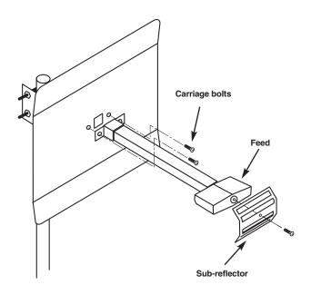
Figure 3-1. Attaching the Sub-Reflector.
