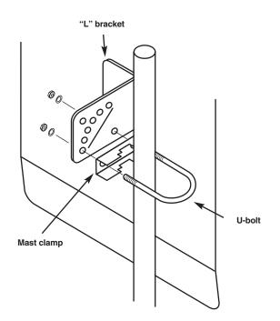
Figure 3-4. Attaching the "L" Bracket.
