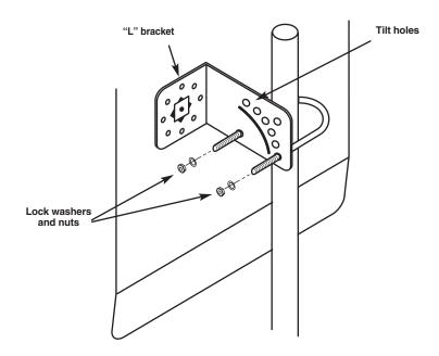
Figure 3-5. Fastening the U-Bolt on the "L" Bracket.
