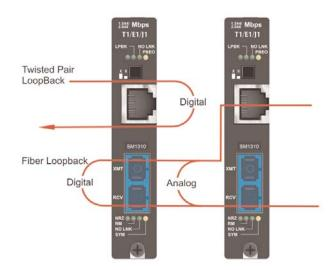
Loopback testing aids in troubleshooting problems with network connections should they occur. "Looping" received data back onto the transmit path helps determine whether a connection is still valid. Twisted pair digital loopback tests isolate problems on the copper run between a T1/E1 converter and the connected device, while fiber digital loopback tests isolate problems on the fiber run.
