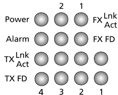
The transmission in full duplex mode is indicated by the related LED (on). If the connection is working in half duplex mode, this LED indicates collisions for the connected segment (flashing).
