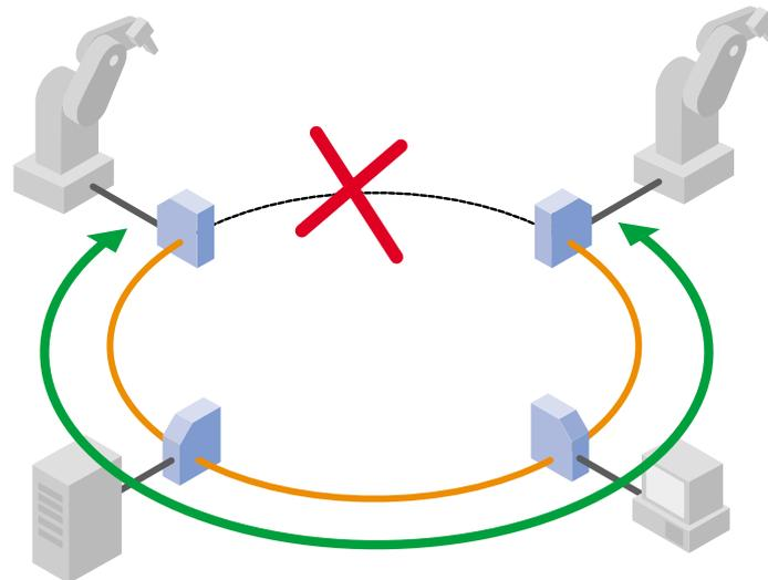
Data transmission in failure status
