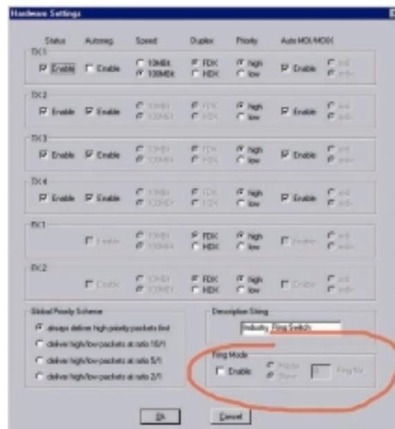
At the menu point Hardware Setting it is possible to select the two modes master or slave. The switch which is configured in master mode is doing the ring manager functions to avoid the multiplication of the data.
