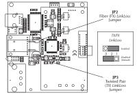
To enable TX or FX LinkLoss, reposition the shunt on the 3-pin jumper indicated over the appropriate pins.
