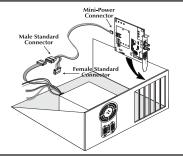
Attach the keyed mini-power connector to PC Media Converter TX/FX. Attach the male end of the "Y" connector to a standard size power connector in your computer. Replace the cover. Attach the cables between PC Media Converter TX/FX and the devices that will be interconnected.
