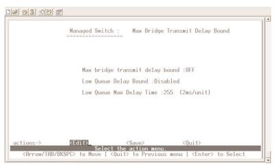
Figure 8-19. Max Bridge Transmit Delay Bound screen.
