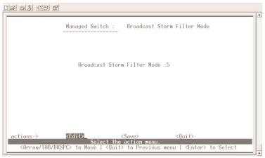
Figure 8-18. Broadcast Storm Filter Mode screen.
