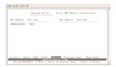
Figure 8-41. Delete Static MAC Address Configuration screen.
