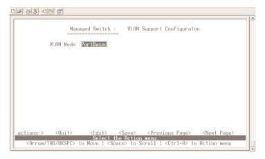
Figure 8-7. VLAN Mode, Port Based.
