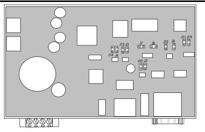
Figure 8. 2 Port Industrial Serial Server Bias Jumper Locations
