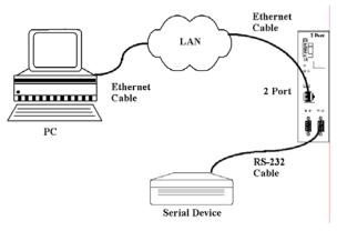
Figure 19. Ethernet Connection via a LAN
