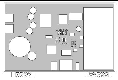
Figure 6. 1 Port Industrial Serial Server Bias Jumper Locations
