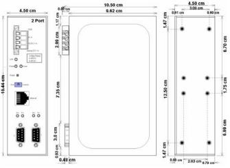
Figure 47. Dimensional Diagram of the 1 or 2 Port Serial Server
