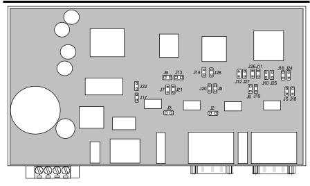
Figure 10. 4 Port Industrial Serial Server Bias Jumper Locations
