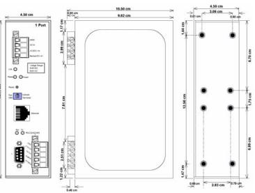
Figure 46. Dimensional Diagram of the 1 or 2 Port Serial Server
