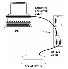
Figure 20. Direct Ethernet Connection using a Crossover Cable
