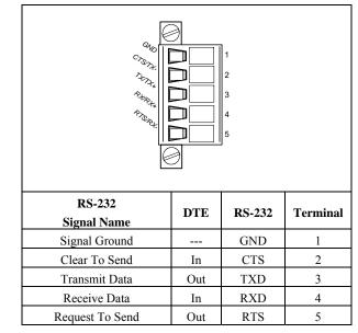
Figure 50. 1 Port Serial Server Terminal Block Pinout in RS-232 Mode
