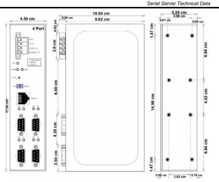
Figure 48. Dimensional Diagram of the 4 Port Serial Server
